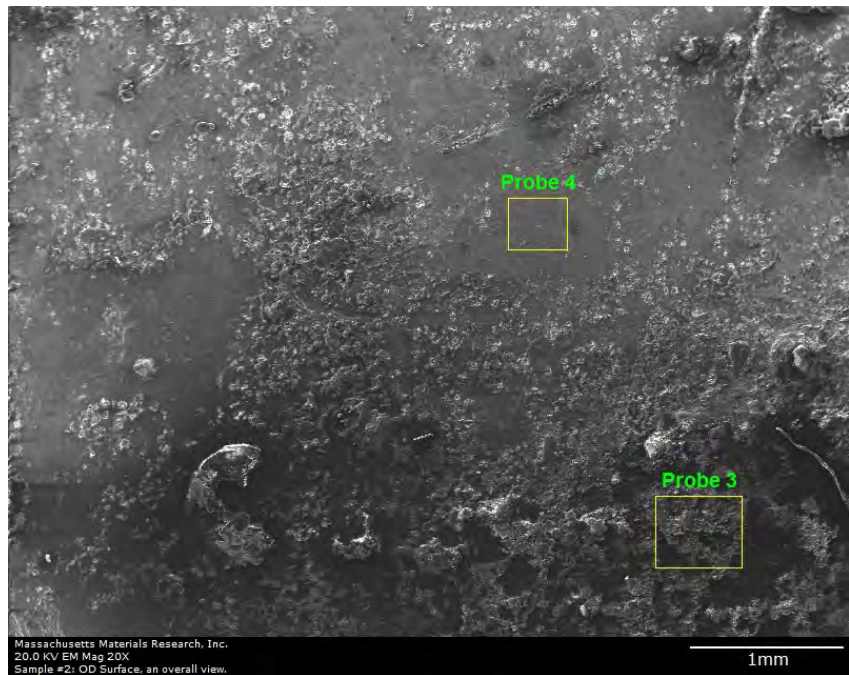
Figure 22: EDS Probes 3 and 4 locations.
