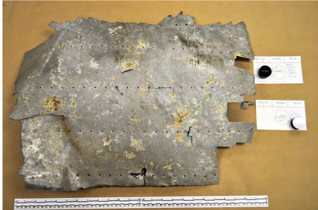
Figure 23: Overall view of metallurgical mount location sources.
