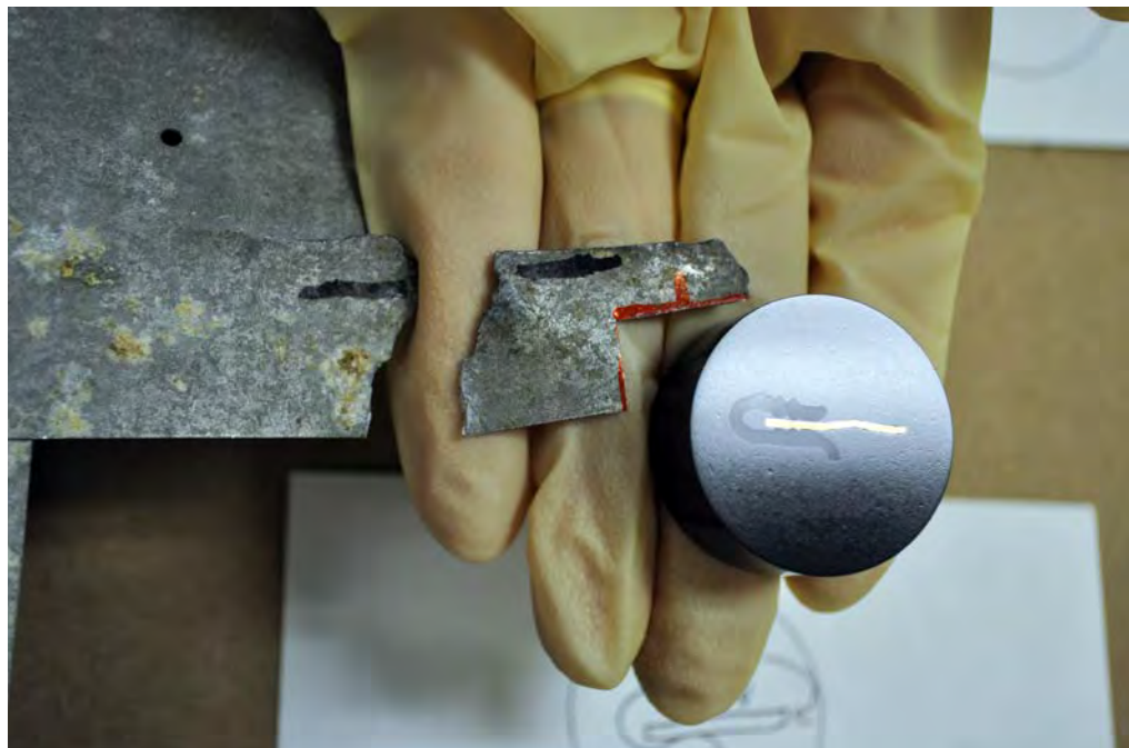
Figure 26: Re-alignment of the separated fragment mount.
