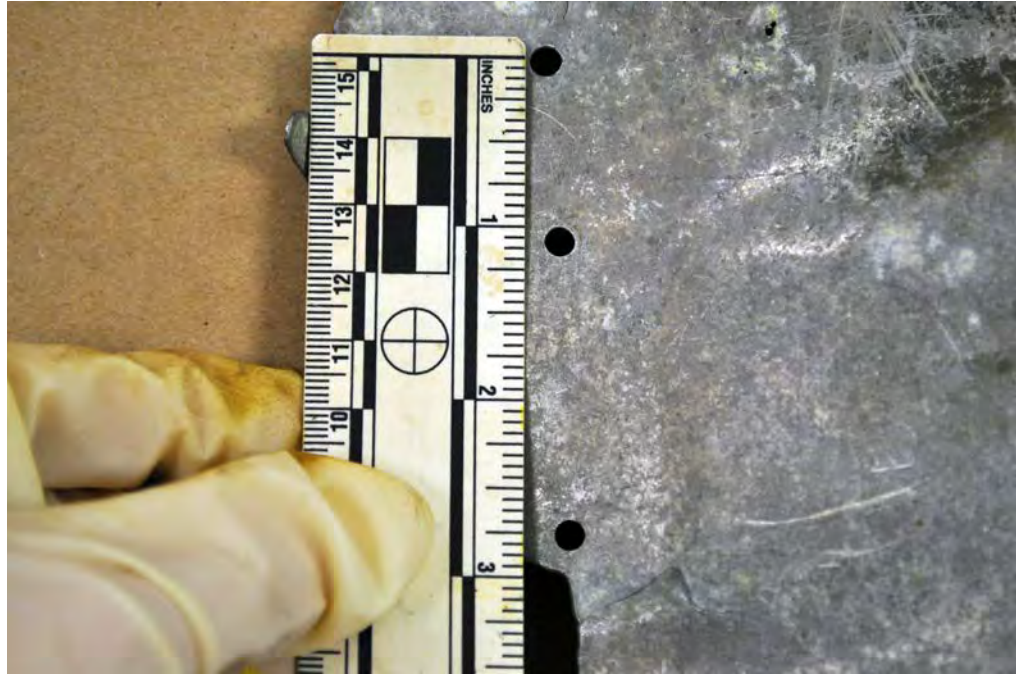
Figure 7: The irregular spacing and linear misalignment of the larger tab rivet holes.
