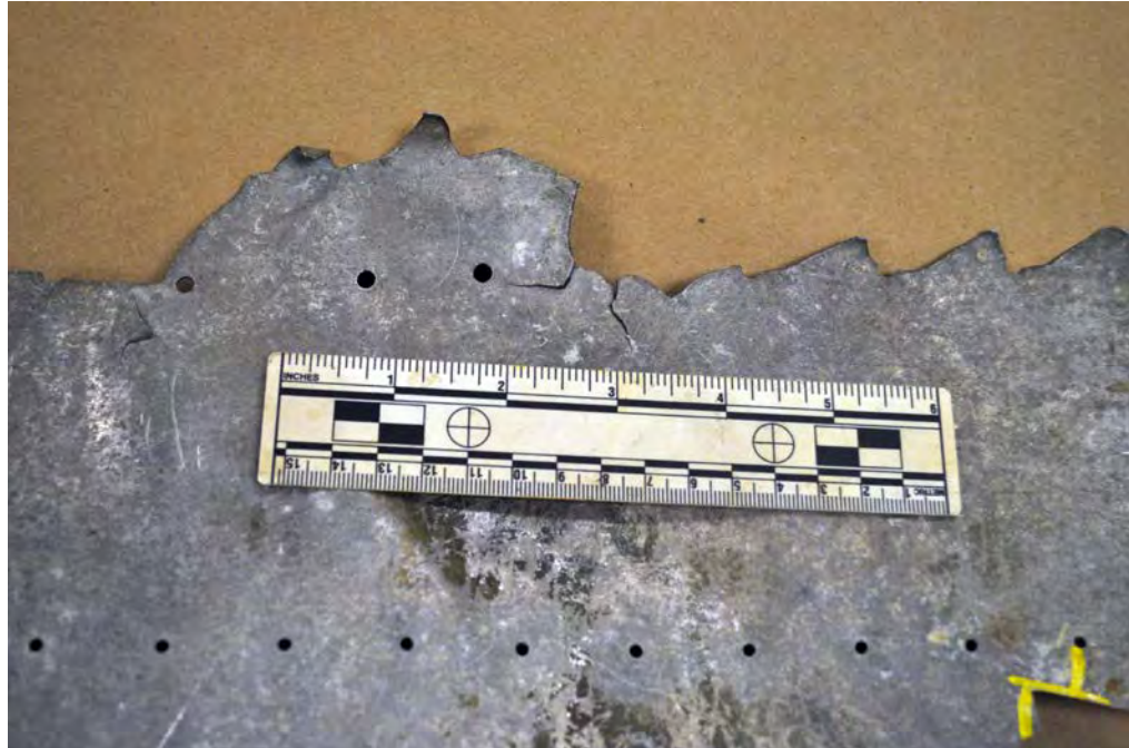
Figure 5: The larger rivet holes remaining on the artifact at the tab feature.
